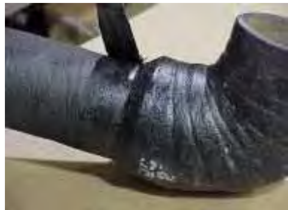
Figure 20 A clean smooth fillet gives the joint a professional appearance.
