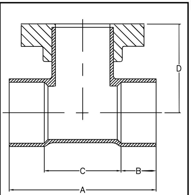
NOTE: DIMENSIONS APPLY TO ALL FLG X SOCKET CONFIGURATIONS.
